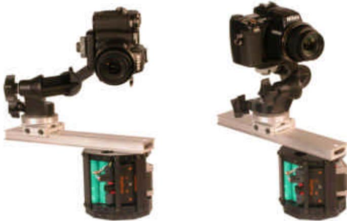
The tripod head supplied is a Bogen 3025, which allows rotation around three independent axes. This combined with the sliding mounting plate allows essentially any camera to be mounted in most any reasonable position, with no camera specific adapter plates required. The pictures above show the camera in both portrait and landscape orientations, with the lens nodal point aligned with the center of rotation.
