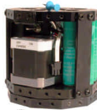
With the switch in the On position, power is applied to the controller, and optionally the camera.
