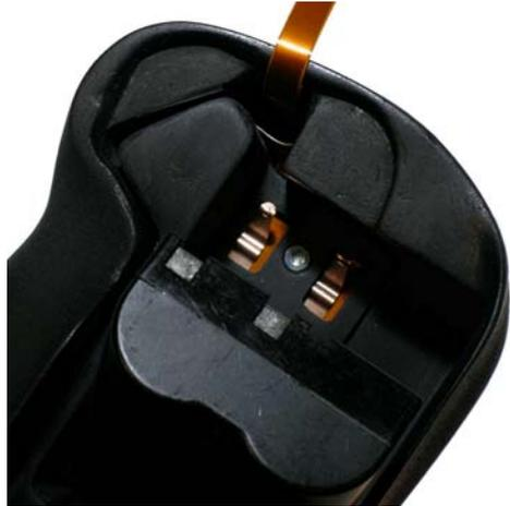
If you use one or two packs, one must be placed upright on the grip, and the tethered battery cap dropped over the end of the battery pack. There are contacts in the cap which mate with the battery pack, and the orientation becomes obvious when you handle it.
